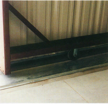
Standard T-Hangar wheels are 6" V-Groove with grease fittings on Inverted Angle Track.
